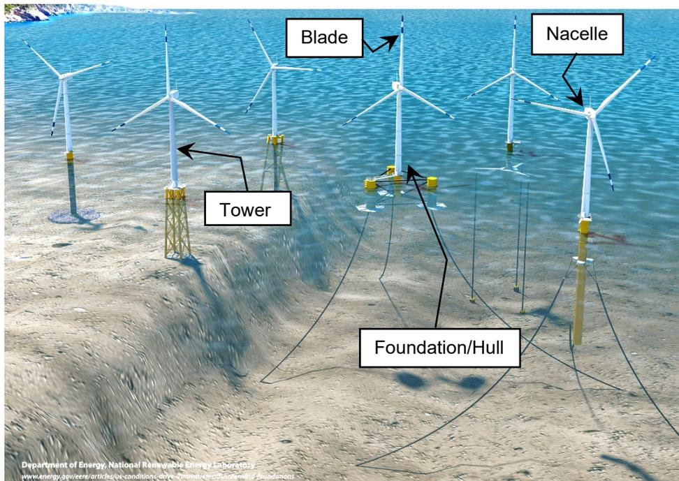
Note that the fixed foundations (at left) are attached to the ocean floor in waters of 200 feet or less. Floating foundations (at right) have emerged as a solution for water depths greater than 200 feet. (Source: NREL)
